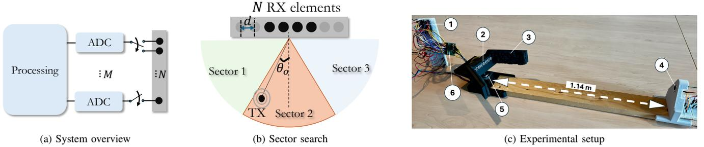
Fig. 1: Fig 1a shows a switched receive array, where  $M$  switches are used to select which of the  $N$  microphones are connected to the  $M$  ADCs. The RX array is first mechanically steered to scan different sectors, as shown in Fig 1b. Then, the DoA within the sector is electronically determined. Our testbed in Fig 1c comprises: 1. Teensy 2. RX array 3. Acoustic barrier 4. TX 5. Stepper motor 6. ADC.
