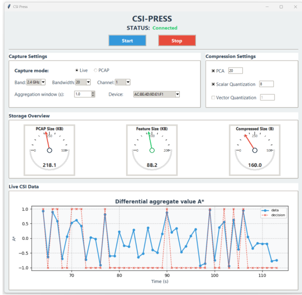
Fig. 2: CSI-PRESS User Interface with a configuration tab, the compression settings, the feature output, and an overview of the instantaneous storage impact.
