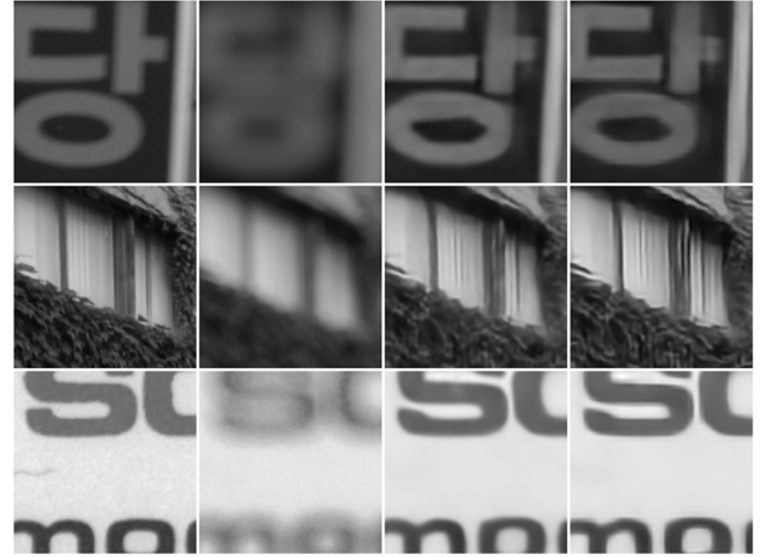
Fig. 4: Comparison of restorations from XY-Deblur on 3 datasets. (L–R) GT image. Blurry image ( \Omega=3.07, 1.47, 1.04 ). Image restored with \mathcal{L}_\varphi ( \Omega=1.34, 1.33, 2.24 ). Image restored with \mathcal{L} ( \Omega=0.79, 2.59, 2.13 ). Models fine-tuned using our composite loss \mathcal{L} produce sharper edges.
