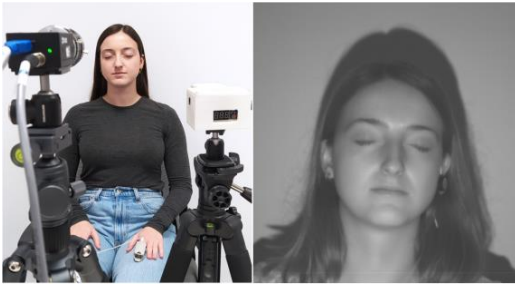
Fig. 1. Experimental setup and example of NIR imaging. The left image shows the experimental setup, including the NIR camera, NIR illumination source, and PPG sensor placed on the subject's index finger. The right image presents an example of a NIR facial image captured during the experiment, demonstrating the imaging conditions and illumination uniformity.
