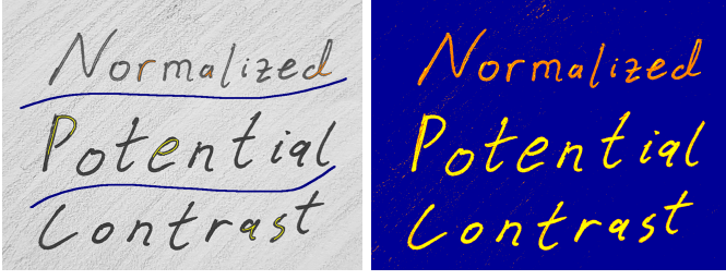
Fig. 2. Left: The example image from Figure 1, now with three different classes labeled. Labels for one ink are in yellow, for a second ink are in orange, and for the background are in blue. Top Right: a multi-class NPC result, where the colors reflect the class segmentation. The multi-class NPC has a value of 0.885.
