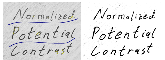
Fig. 1. (Left) An example image, where labeled background pixels are shown in blue and labeled foreground pixels are in yellow. (Right) The binarization resulting from potential contrast, with a value of 254.983 for an 8-bit image, and a normalized potential contrast value of 0.996.
