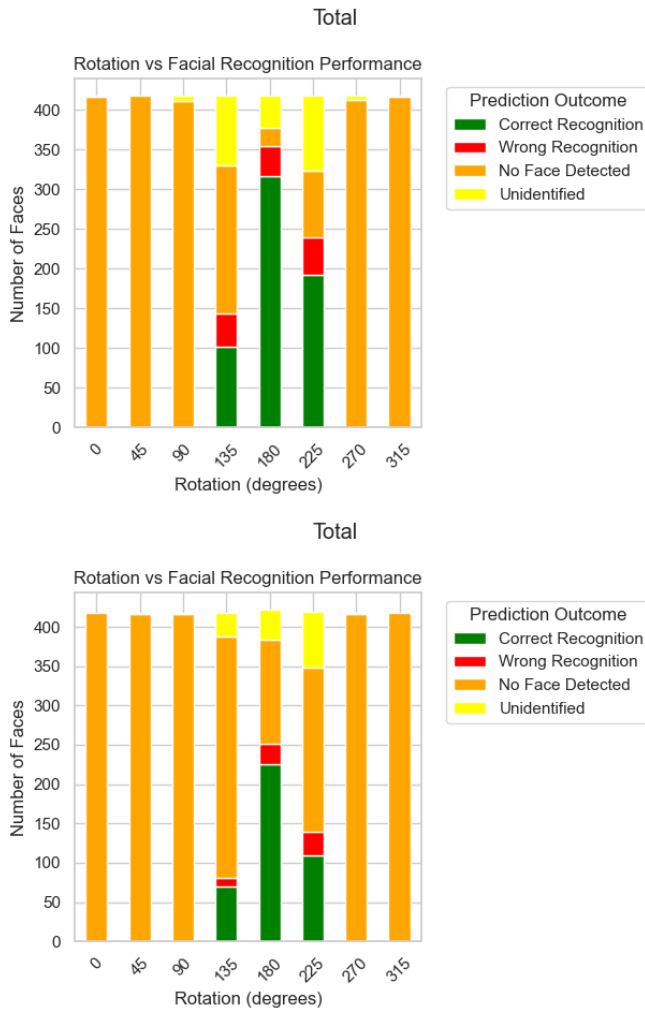
Fig. 3: Face recognition results in bright (top) and Dark (bottom) lighting conditions
