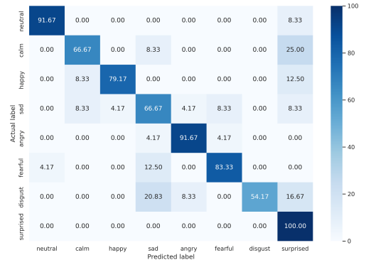
Fig. 4: Confusion matrix of the results of multi-channel Sum PE MER model on RAVDESS test set convolved with ACE Lecture Room 2 ( T_{60} = 1220 ms).
