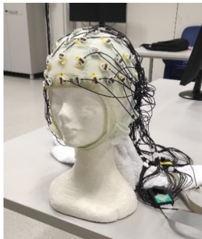
Fig.1. Positioning of the electrode cap on the mannequin. A wet towel was placed between the head of the mannequin and the EEG cap to mimic the conductivity of the human skin.
