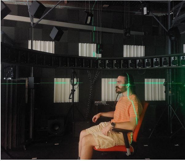
Fig. 2: HRTF measurement setup.
