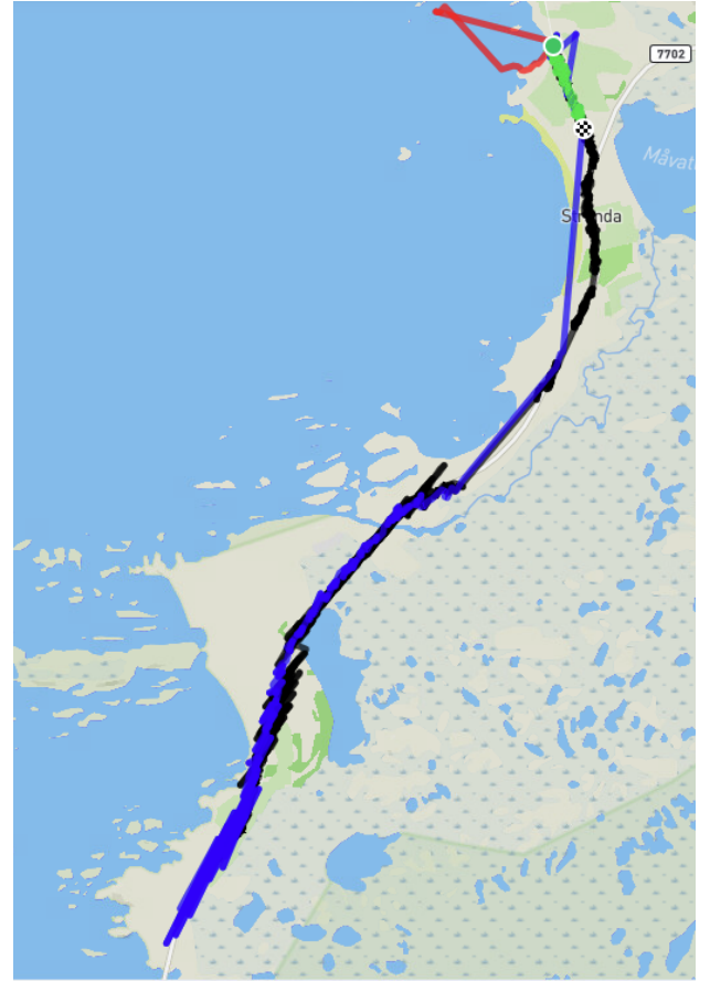
Fig. 3: The receiver positions for the authentic GNSS navigation (the reference trajectory in black), the spoofed receiver (in red), the PI-STAP (in green) and the LC-STAP (in blue).
